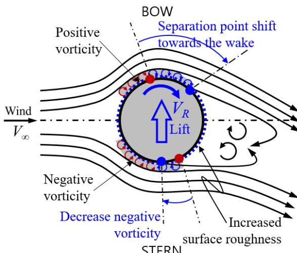
Fig. 13 Improved Magnus effect by increasing surface roughness
