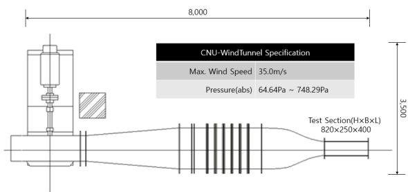
Fig. 2 CNU Wind Tunnel
