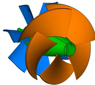
Fig. 12 3-dimensional shape of the re-designed waterjet propulsor (WJ-II)
