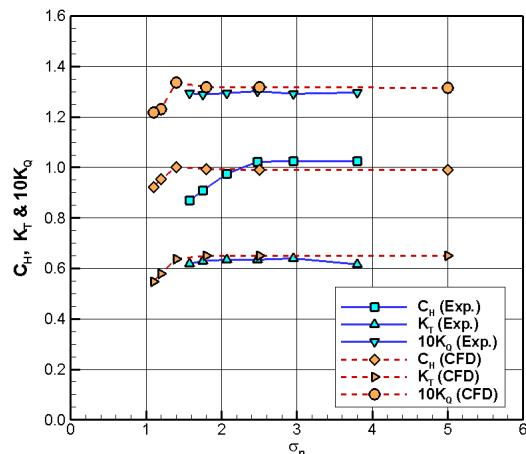
Fig. 11 Variation of head, thrust and torque coefficients with respect to cavitation number for the waterjet propulsor, WJ-I
