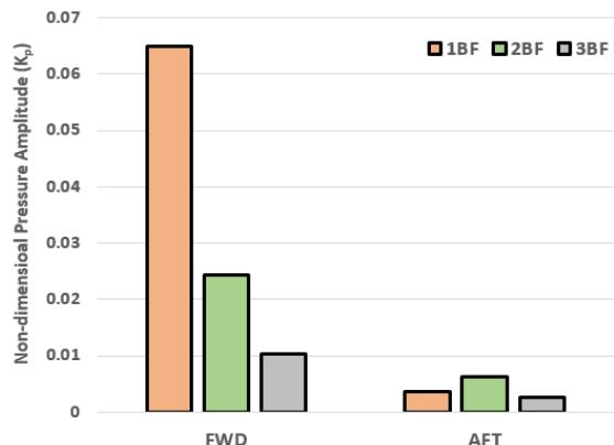
Fig. 15 Calculated non-dimensional fluctuating pressure amplitudes (WJ-II)
