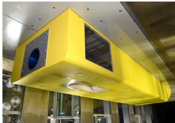
Fig. 1 Vehicle model installed in the test section of LCT
