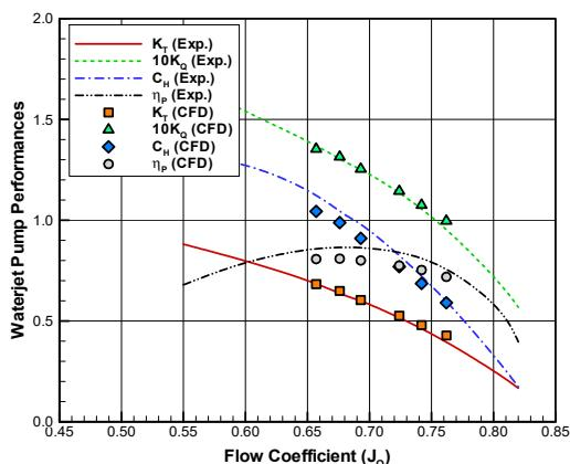
Fig. 8 Comparison of waterjet pump performances (WJ-I)
