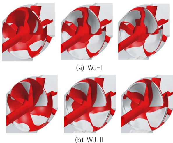
Fig. 13 Comparison of calculated cavity patterns on the waterjet impeller blade (Left:  $\sigma_n=1.8$ , Middle:  $\sigma_n=1.4$ , Right:  $\sigma_n=1.2$ )
