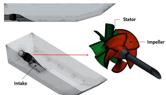
Fig. 4 Surface grid of the model vehicle and waterjet propulsor
