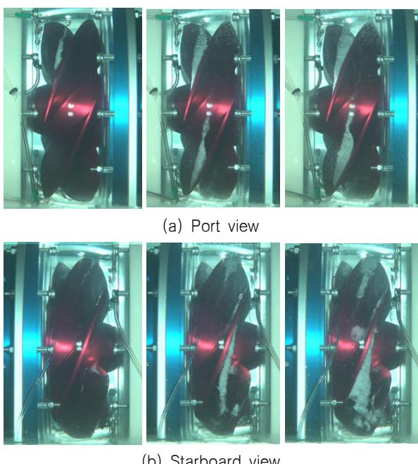
Fig. 9 Observed cavitation patterns for the waterjet propulsor, WJ-I (Left:  $\sigma_n=2.5$ , Middle:  $\sigma_n=1.8$ , Right:  $\sigma_n=1.6$ )
