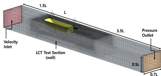
Fig. 3 Computational domain for the waterjet analysis
