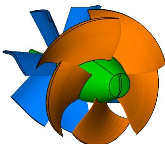
Fig. 7 3-dimensional shape of the waterjet propulsor (WJ-I)
