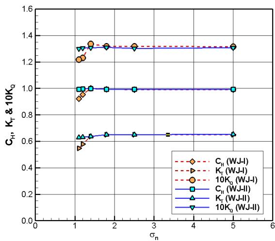
Fig. 14 Comparison of head, thrust and torque coefficients with respect to cavitation number for the waterjet propulsors, WJ-I and WJ-II
