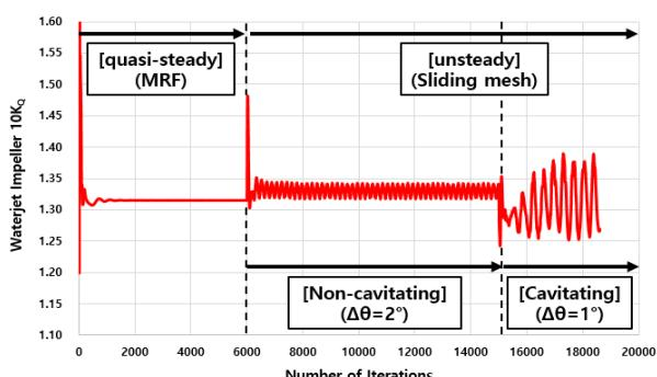
Fig. 6 Computing procedure for the waterjet cavitating flow
