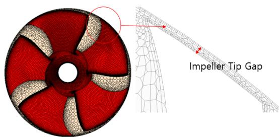
Fig. 5 Grid system around the waterjet impeller blade and tip region
