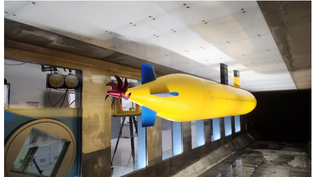
Fig. 3 Installation of the model submarine with E1619O inside the test section of the large cavitation tunnel
