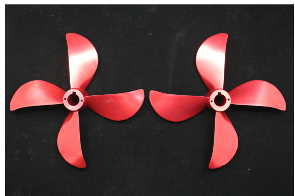
Fig. 8 Model propellers (Left : KP1800 / Right : KP1801), inward rotation viewed from downstream
