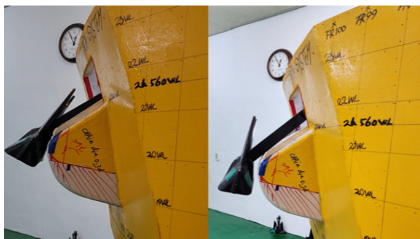
(a) Interference and folding check between bolster and anchor
