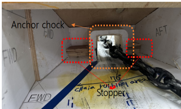
(c) Anchor chock and stopper mock up
