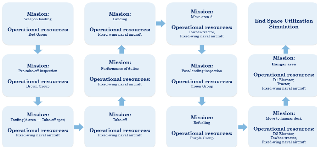
Fig. 7 Discrete event simulation process for space utilization simulation using SimPy
