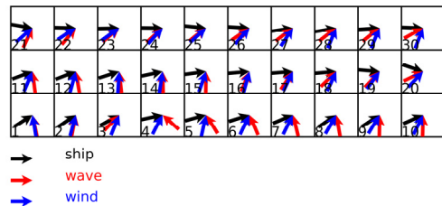
Fig. 16 Relative wind and wave direction of way points from Busan to PR
