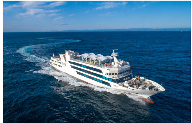
Fig. 1 2,700ton-class electric propulsion smart ship (ULSAN TAEHWA)
