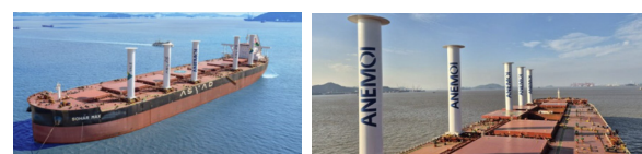
Fig. 1 Rotor sails installed on the VLOC (Source: Hakirevic Prevljak, 2025)
