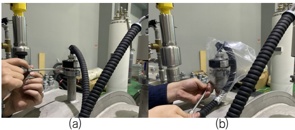
Fig. 3 Helium leak test method (a) probe method and (b) hood method.
