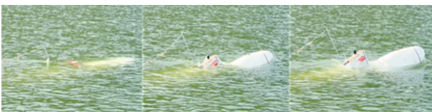
Fig. 6 Surfacing after depth control tests
