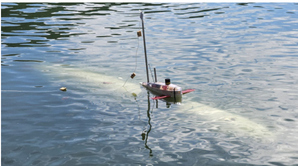
Fig. 4 BB2 model in snorkel-ready condition
