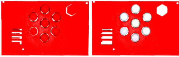
(a) distance_threshold : 0.05 (b) distance_threshold : 0.01 Fig. 13 Plane recognition results of test board point cloud according to RANSAC algorithm
