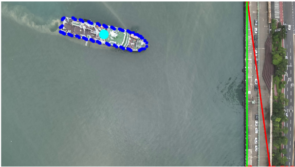
Fig. 8. Quay wall line detection results using two methods (Red: Method 1 - RANSAC; Green: Method 2 - Dimensionality Reduction)
