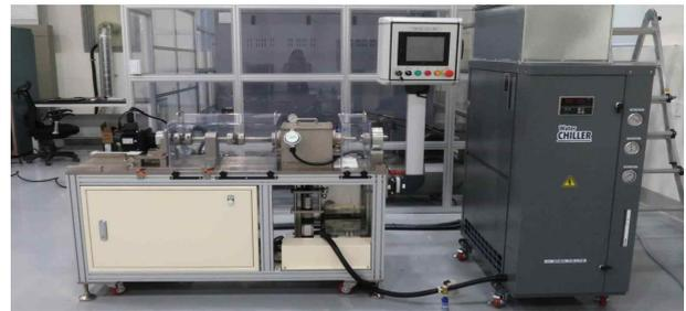
Fig. 3 Equipment of wear resistance test of water lubrication bearing
