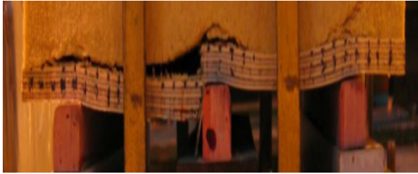
Fig. 2 Failure due to shear in the bottom plywood of the panel (Lee and Kim, 2006)
