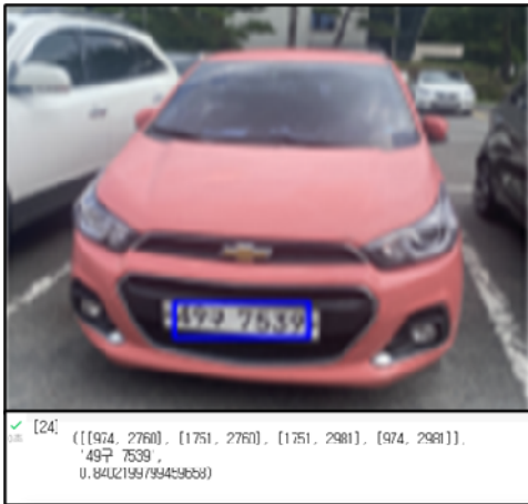
Fig. 5 Recognition of license plate using EasyOCR
