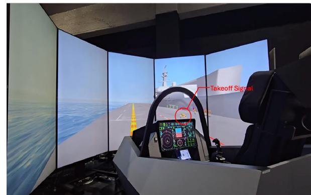
Fig. 18 STOVL take-off seen from the cockpit mockup
