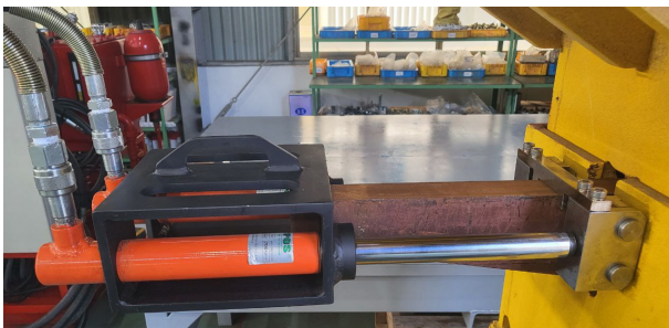
Fig. 18 Block support height adjustment performance evaluation
