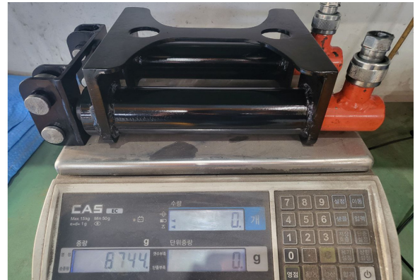
Fig. 23 Weight of the prototype of the redesigned block support height adjustment device
