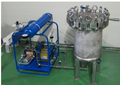
Fig. 11 Pressure chamber for watertightness test
