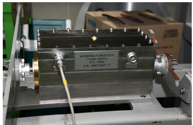
Fig. 6 Torque sensor including encoder
