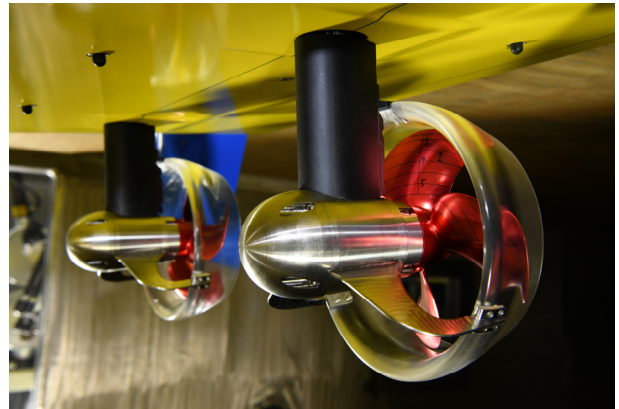
Fig. 2 Azimuth thruster composed of propeller, duct and pod
