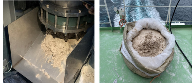
Fig. 10 CaCO 3 discharged from the bottom of the Solid-liquid separator
