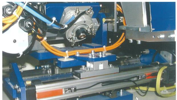
Fig. 9 AS-Interface actuator on rotary index table
