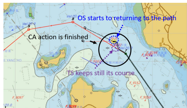
(c) OS starts to returning to the path and TS keeps still its course Fig. 16 The one of the CA actions during simulation
