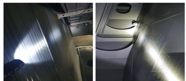
(a) Deformation check using light
