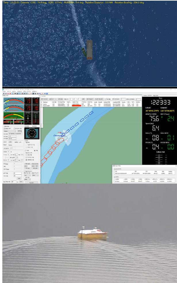
Fig. 21 3D(upper)/2D(mid) view of the RESCA and the CCTV view(lower) of free running model test at the collision time of replay of ships colliding accident(Case 2)
