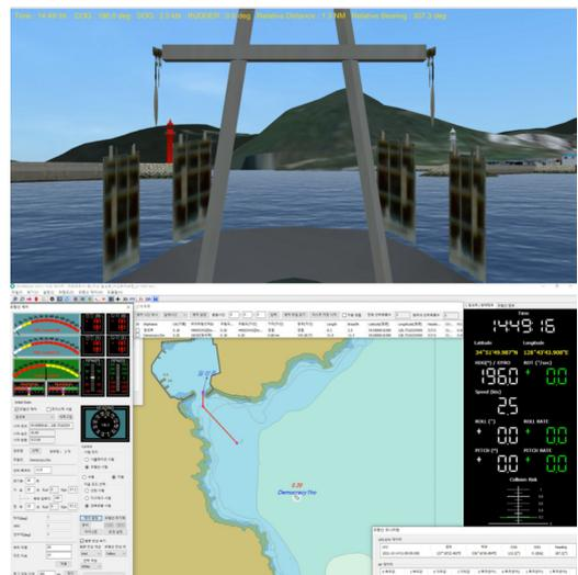
Fig. 4 View of RESCA (Above: 3D, below: 2D(ENC: Electronic Navigational Chart))
