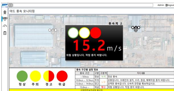
Fig. 22 Wind speed visualization screen(anemometer 2)
