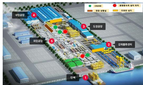
Fig. 13 Equipment layout for wind speed monitoring
