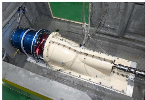
Fig. 2 Waterjet propulsor model inside the vehicle model
