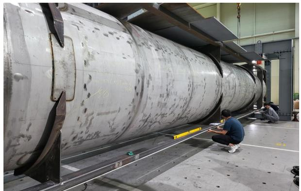
Fig. 19 Measurement of longitudinal displacement
