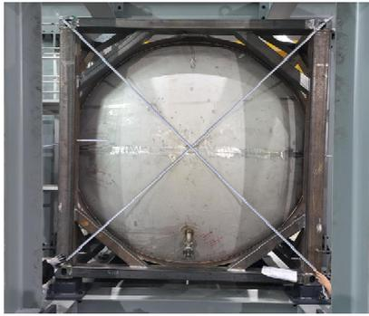
Fig. 20 Measurement of end wall diagonal dimensions
