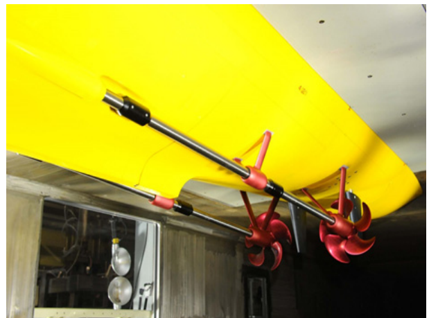
Fig. 6 The stern appendages installed on the model ship
