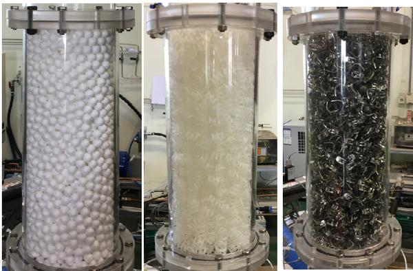
(a) Packed bed (Sphere) (b) Pall ring type (PP) (c) Saddle type (STS)
