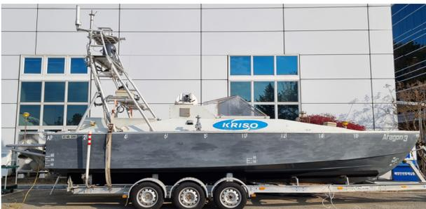
Fig. 1 USV Aragon3 with waterjet propulsion system
