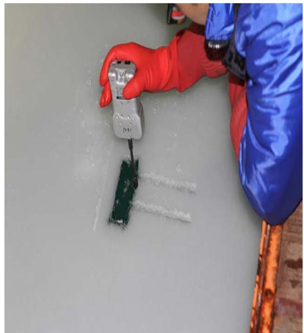
Fig. 3 Flexural strength measurement process by cantilever beam test (Jeong and Ha, 2020)
