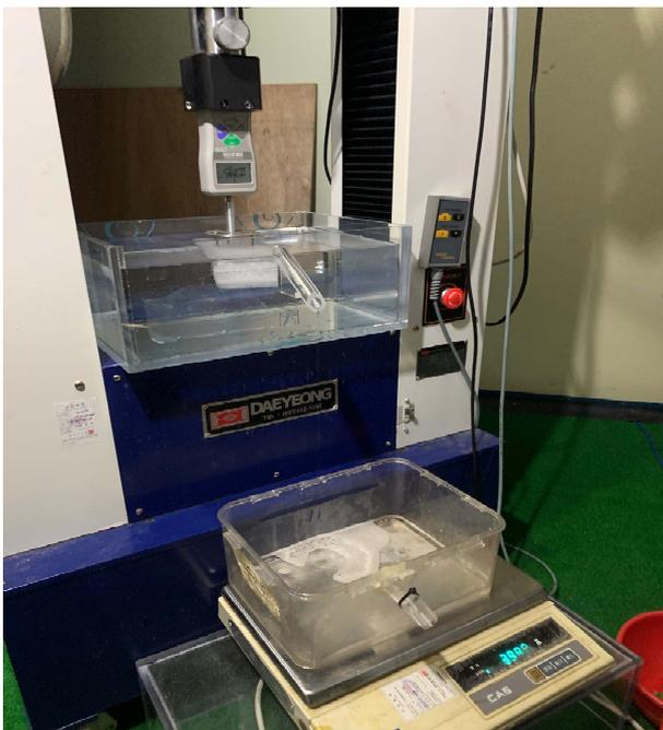
Fig. 2 Density measurement process by displacement method
