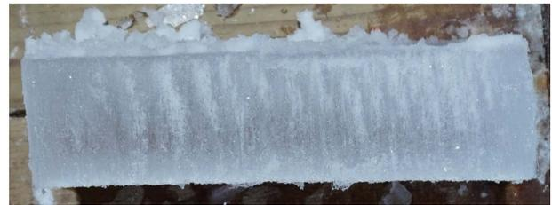
Fig. 6 Side view of a model ice specimen w/o micro-bubble
