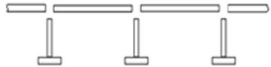
Fig. 8 A plate-stiffener separation model
