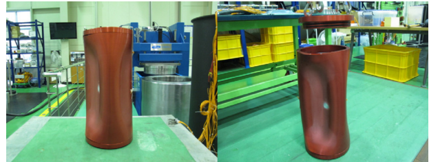
Fig. 6 Collapse of thick cylinder (Choi, et al., 2016)
