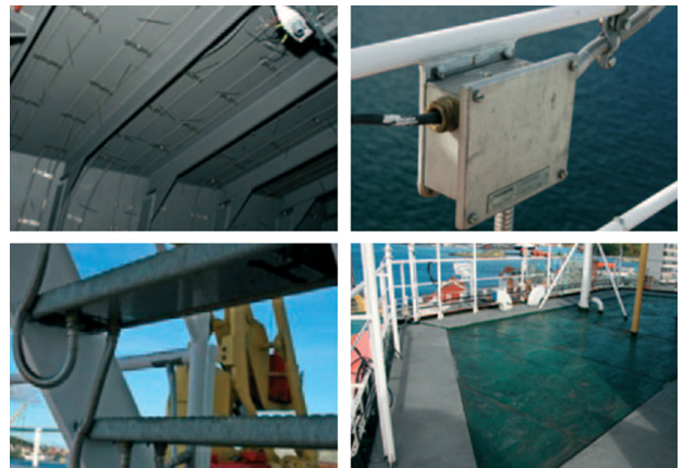
Fig. 7 Winterization methods of deck machinery(URL: http:// www.tranberg.com )
