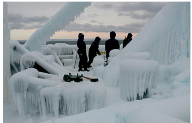
Fig. 2 Icing on deck and ice removal process by vessel crews(URL: http://www.groupocean.com )
