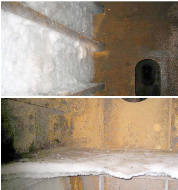
Fig. 17 Freezing of ballast tank water(Upcraft, 2008)
