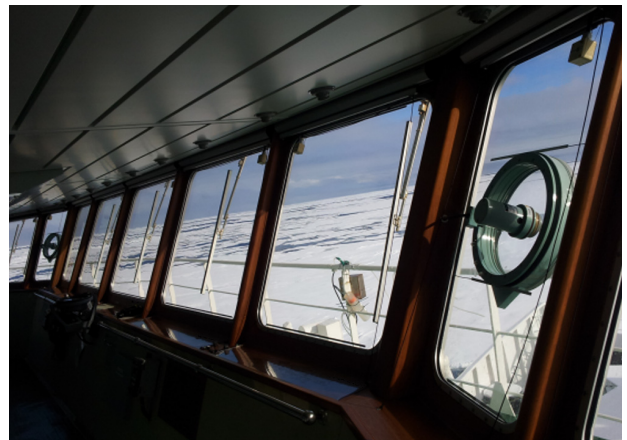
Fig. 6 CVS and window wiper installed on icebreaker Araon
