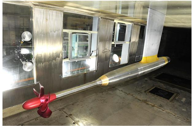
Fig. 4 Submerged body & strut for inclined-shaft dynamometer
