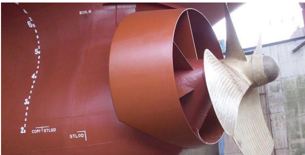
Fig. 2 Becker Mewis Duct
