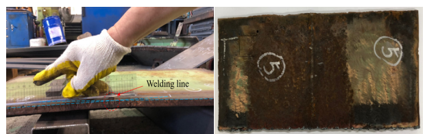
Fig. 2 Bending deformation and corrosion damage of aged steels
