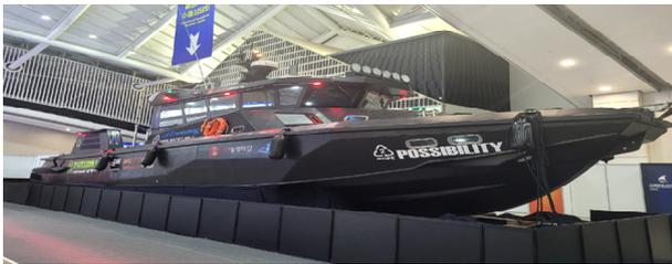
Fig. 1 HDPE power boat prototype
