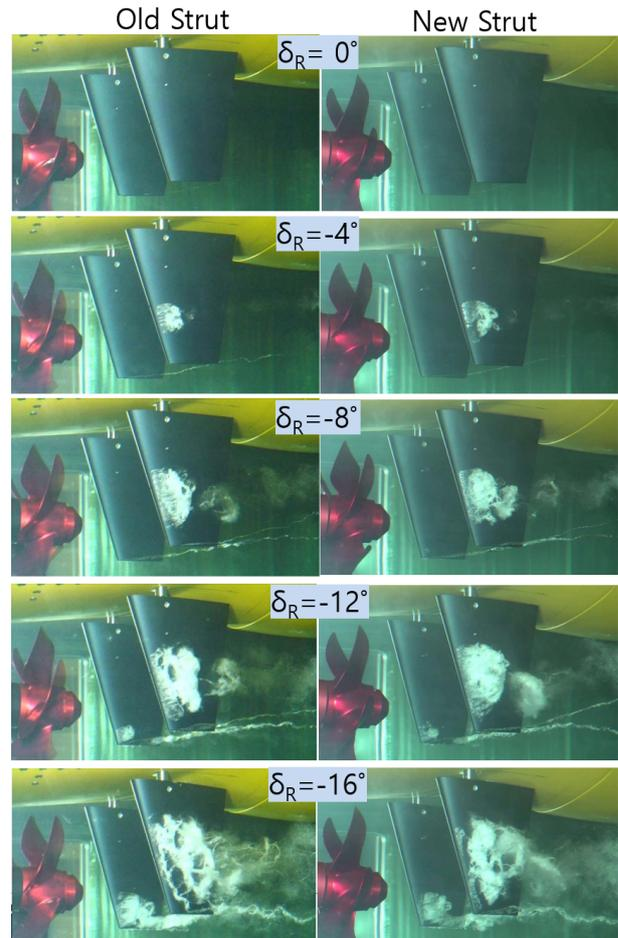
Fig. 14 Rudder cavitation at behind old & new struts
