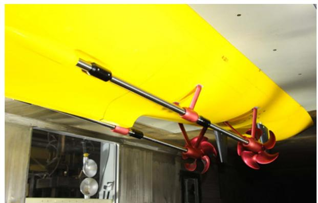
Fig. 2 The stern appendages installed on the model ship
