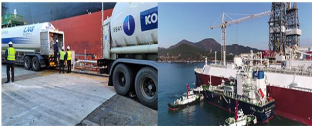
Fig. 2 Example TTS & STS LNG bunkering (KOLB, 2022)
