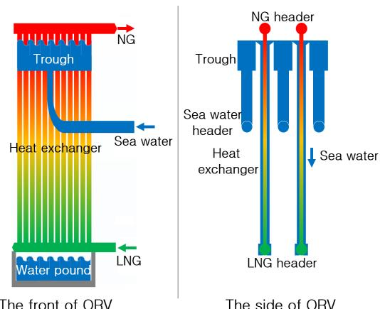
Fig. 1 Structure of an open rack vaporizer
