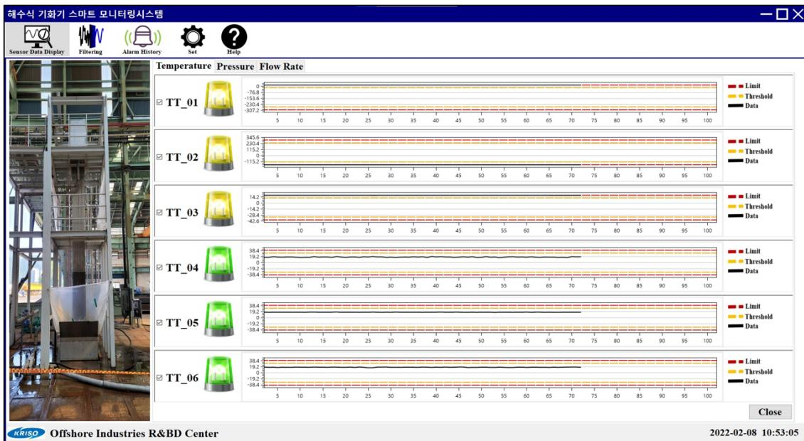
Fig. 7 Implementation results of the monitoring system – sensor data display view
