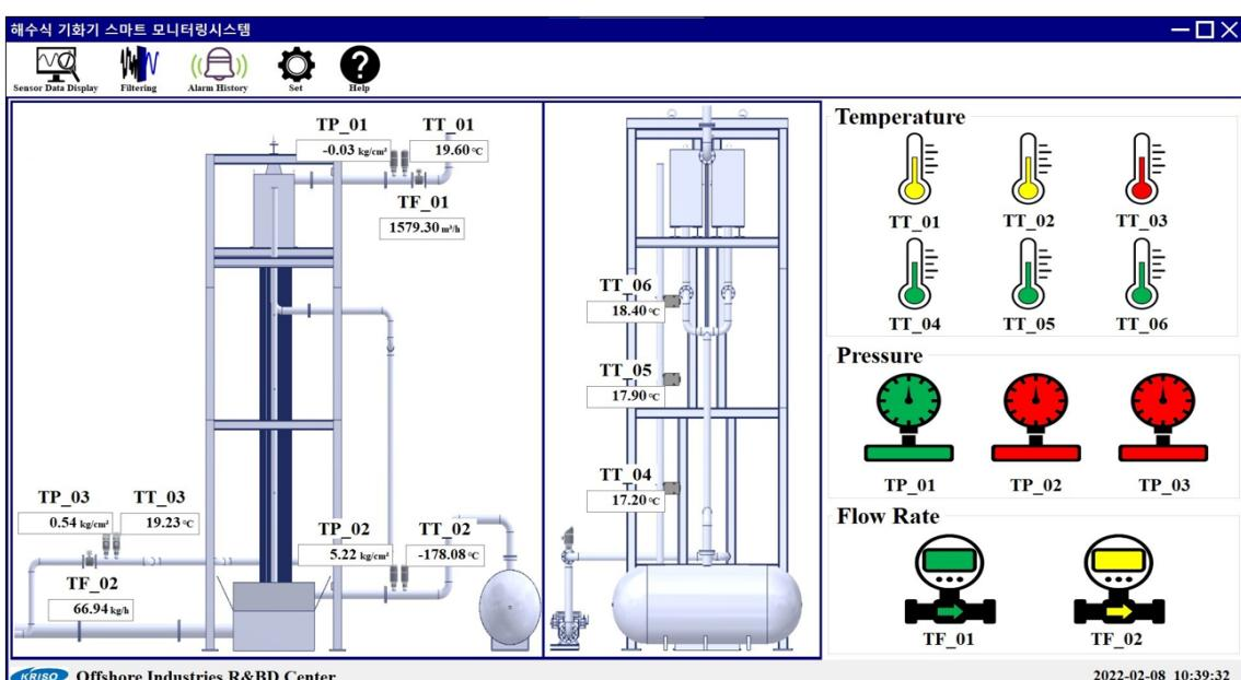
Fig. 6 Implementation results of the monitoring system – main view
