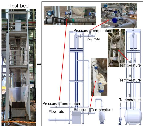
Fig. 2 Location of sensors installed test bed
