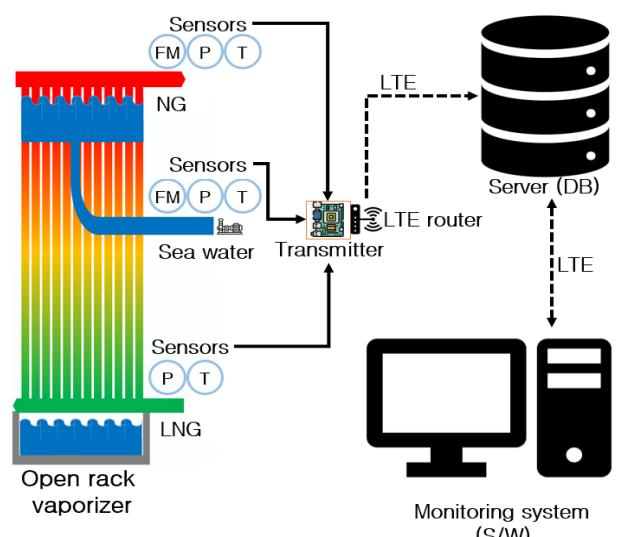
Fig. 3 Construction of infrastructure for operation state monitoring system for open rack vaporizer
