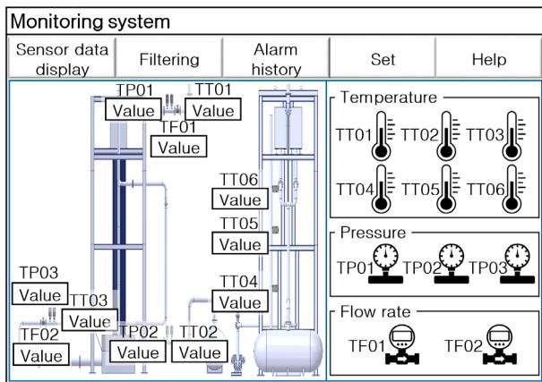
Fig. 5 Graphical user interface for the monitoring system – main view
