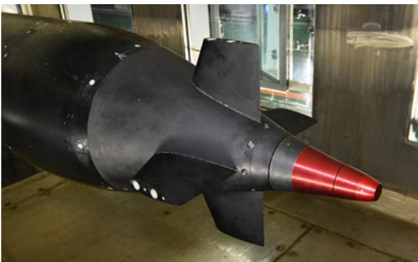
Fig. 5 Setup for bare hull resistance test
