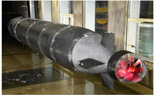
Fig. 9 Installation for the self-propulsion test
