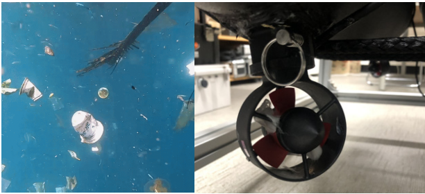
Fig. 2 (Left) Marine debris, (Right) Propeller failure due to the Marine debris
