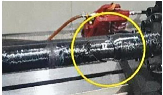
Fig. 14 Tube failure of 1/20 scaled CFRP shaft
