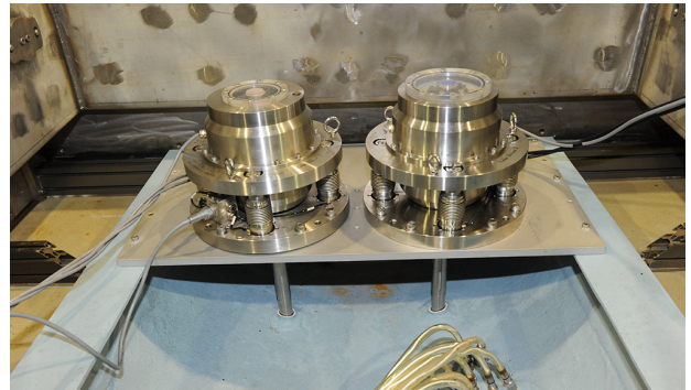
Fig. 2 Rudder dynamometers installed on the model ship
