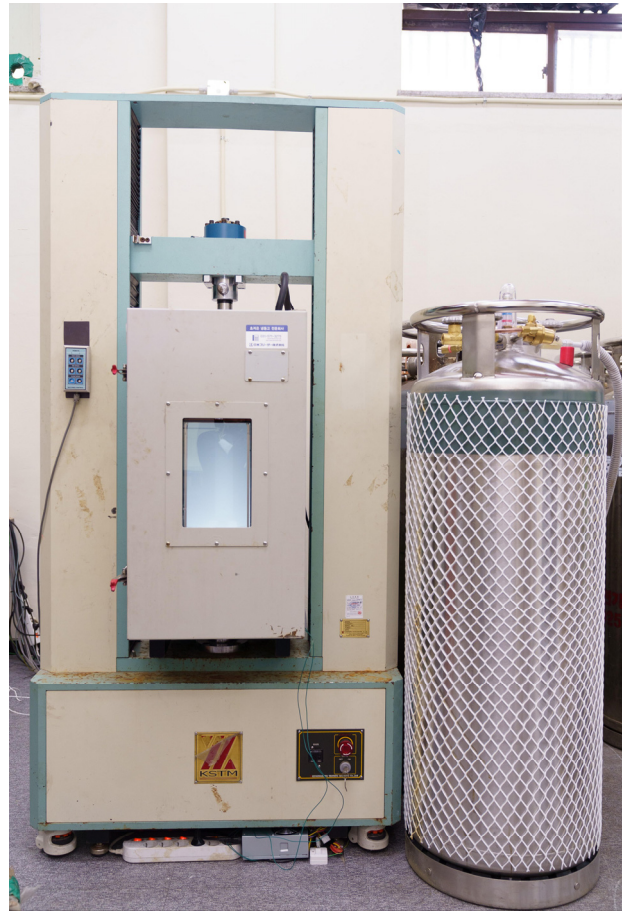
Fig. 5 UTM with cryogenic chamber and Liquid nitrogen
