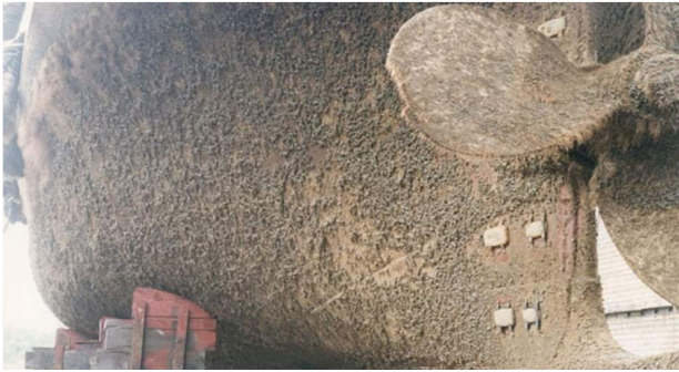
Fig. 20 Ship hull showing extensive fouling by barnacles ( https://www.european-coatings.com/Homepage-news/Nanotechnology-and-anti-fouling )
