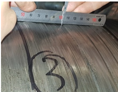
Fig. 4 Propeller shaft damage
