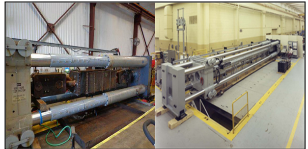
Fig. 11 High load fatigue test machine in overseas center
