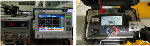
Fig. 16 Conductor resistance & insulation resistance
